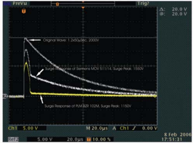
Surge Response of Siemens MOV 511/14 and HVM BZR 102M on 1.2x50µs, 2000V Surge
